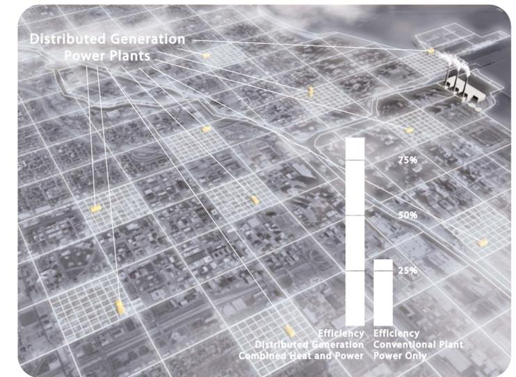
**Tomorrow:** Expanded use of Distributed Generation (DG) power plants generate electricity on site or in a facility located near customers. Since the power is being produced in close proximity to customers, the excess heat created is also available to meet local thermal energy needs. This type of cogeneration or Combined Heat and Power (CHP) application would supply both electricity and thermal energy directly where it is needed.
